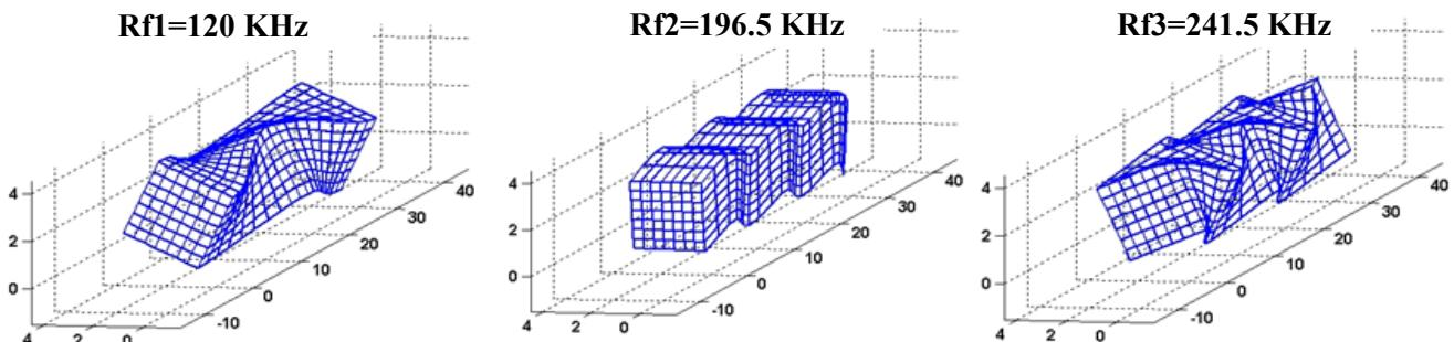
Comparison of temperature dependencies of the measured and calculated resonance frequencies reveals reliable method for identification of vast majority of the experimentally measured resonance modes. It should be emphasized that amplitudes of the experimentally measured piezoelectric resonances strongly differ from each other and mathematical criteria for theoretical analysis of intrinsic vibration mode amplitudes aren't devised so far.
